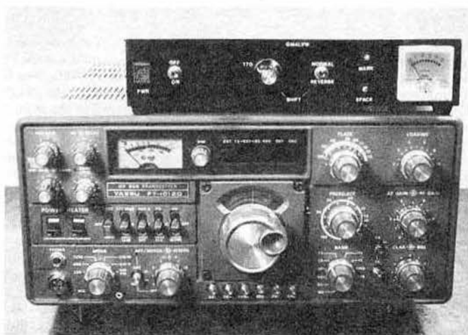
Fig 1. RTTY hardware. A home-made terminal unit surmounting a standard ssb transceiver
